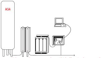
2-metre high pressure hose, MR-60 regulator with inlet filter, signal manometer for connection to the alarm system, shut-off valves and a spanner. The cabinet is designed for outdoor installation. The connection to the alarm system must be well protected (Eexi).
