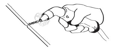
Fig 8. Local extraction on welding gun.
