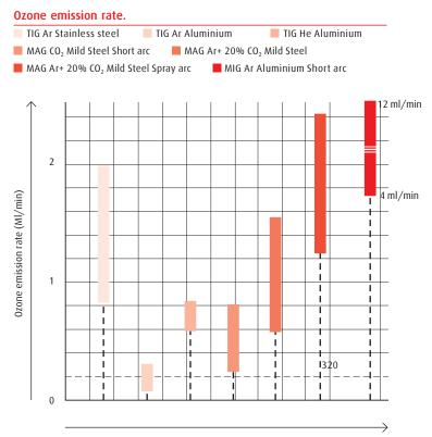
Fig 6. Emissions of ozone measured during welding trials in a laboratory (4).
