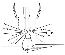
Fig 1. Sources of fume gas metal arc welding (2). 1. Droplet at of wire or during transfer. 2. Weld pool. 3. Electrode spots and anode). 4. Exploiding wire. 5. Large particles. 6. Fine metal droplets ejected by wire explosion.
