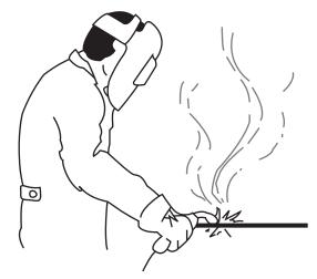
Fig 11. The welder should keep his head outside of the rising plume of air pollutants.
