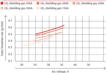
Fig 4. Effect of current and arc voltage on fume emissionin MAG welding of mild steel using carbon dioxide as the shielding gas (3).
