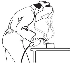
Fig 2. Rising plume of fume and gases from weld spot.
