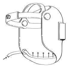
Fig 10. Welding helmet with supply of fresh air.
